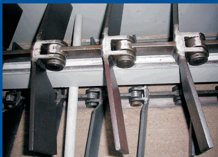
traversini autocentranti sagomati a "V" self-aligning "V-shaped" flights
